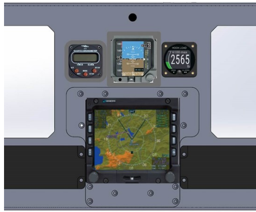
Fig. 4.24 Multi-Functional Displays (MFD) Installation in Instrument Panel
