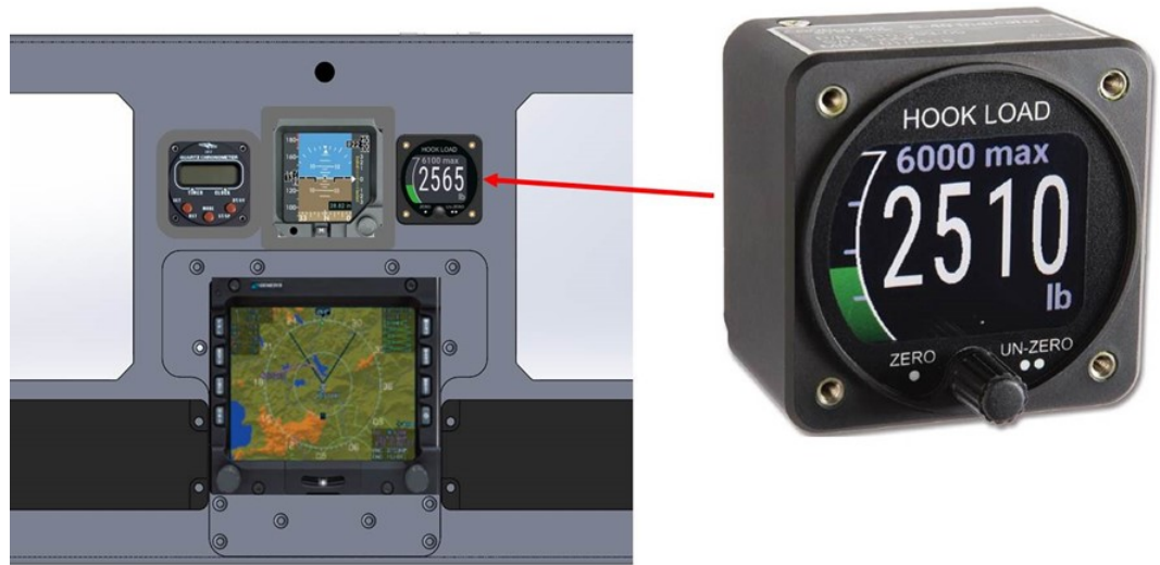
Fig. 4.39 Cargo Hook Display Installation
