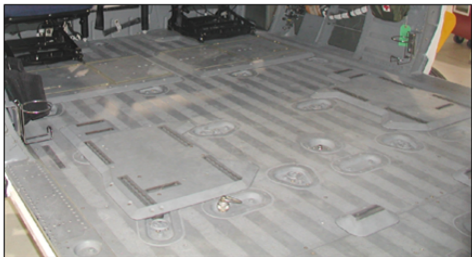
Fig. 4.34 Floor Pallet Installation
