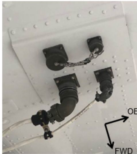
Fig. 4.3 Tank A Kit Electrical/Controls Belly Connector
