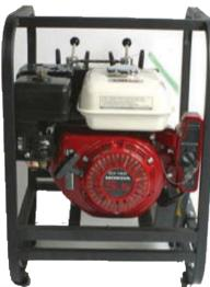
This pump features two tool connections and two tool simultaneous use.
