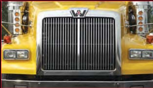
Replaceable vertical grille bars
