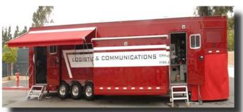
ECC 'B' building at the RFOTC campus to enable it to receive 9-1-1 phone calls. Emergency responses are dispatched via radio. The trailer must be in close proximity (< 50 feet) to the ECC 'B' building to connect to the 9-1-1 phone system. The LCT does not have true emergency dispatch capabilities as it requires a physical connection to the RFOTC Data Center, nor can dispatchers use the OCFA CAD system that is used in the OCFA ECC.
