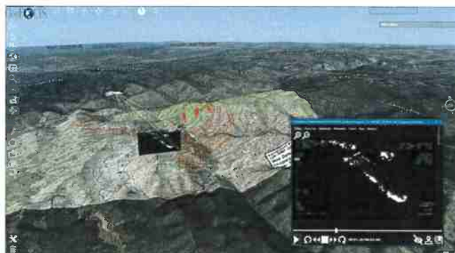
Figure 1. GeoFOCIS 3D Live FMV Projection onto Incident Map GeoPDF.
