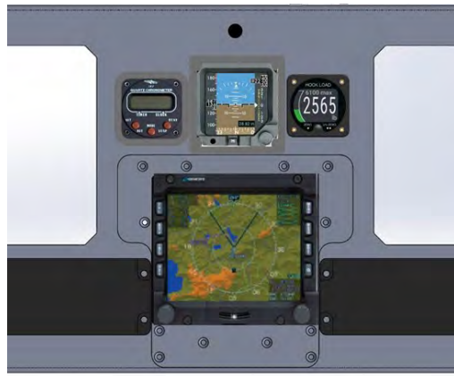
Fig. 4.24 Multi-Functional Displays (MFD) Installation in Instrument Panel
