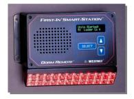
The legacy station alerting systems currently utilize electro-mechanical relays and amplifiers, and will be upgraded with the digital electronic SmartStation, extending the alerting systems' useful life by 15 or more years. The cost per fire station upgrade varies substantially depending on the size of the fire station, number of crew, and apparatus that are deployed. The average cost for the 44 fire stations upgraded to date is approximately \$103,000. When a new fire station is constructed,
