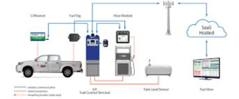
Implementation of this module will improve accountability for fuel utilization, provide pump control and fuel card lockout, and result in overall fuel consumption savings.
