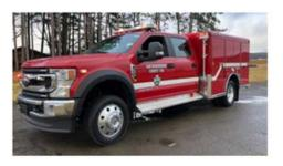
The old US&R support is repurposed squad from the Reserve Program. US32 has multiple mechanical issues and can be unreliable. The new squads are purpose built to meet the needs of the Technical Rescue Program including increased storage, four-wheel drive, higher ground clearance, and easier turning radius.
